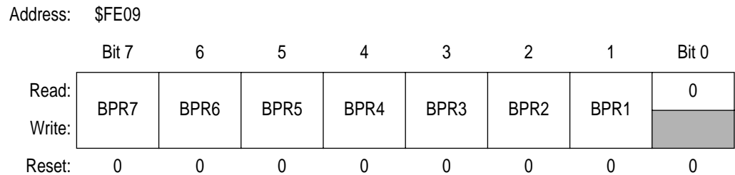
Figure 4-3. FLASH Block Protect Register (FLBPR)
